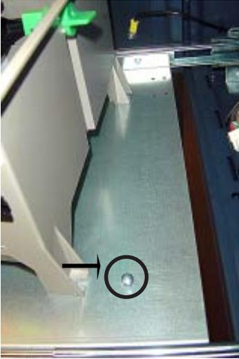
*Figure 4. Align slots of dispenser under screws.*
