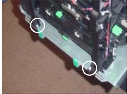
*Figure 5. Install front mounting screws.*
