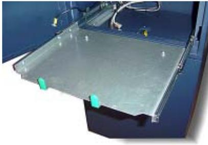
↳ Locate the locking slide tabs on each side of the slide rails. Push tabs up/down on each side and remove tray from rails. Push rails back into cabinet and set tray aside.
