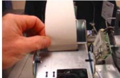
Figure 6-4. Paper/spool in bracket. Figure 6-5. Feed paper in take-up slot.
